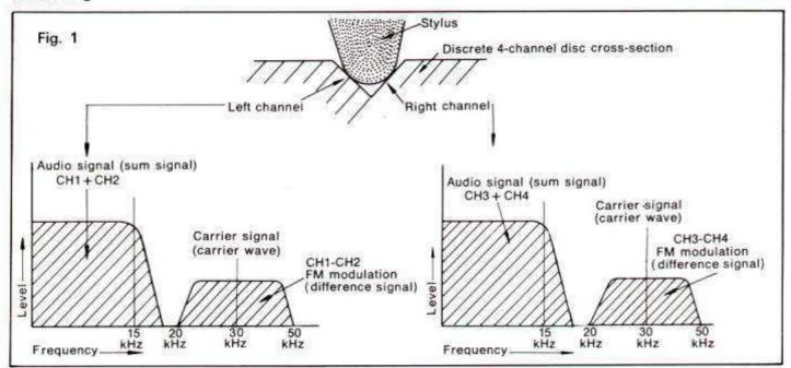
The following is a brief explanation of how four sounds, each independent of the other, are obtained from one groove of a disc.
